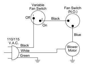
Figure 53 - Blower Wiring Diagram for Thermostat-Controlled Models
